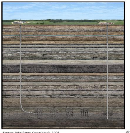
**Contrasting Horizontal and Vertical Drilling**
